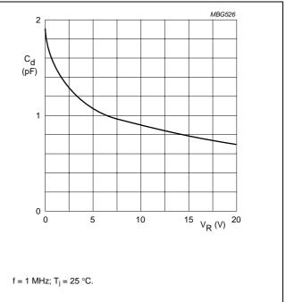
Fig.6 Diode capacitance as a function of reverse voltage; per diode; typical values.
